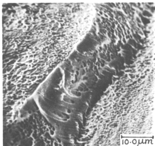
Figure 3 Zr–1.9 wt% Cr, beta quenched. The density of microvoids is smaller in the facet running diagonally.
